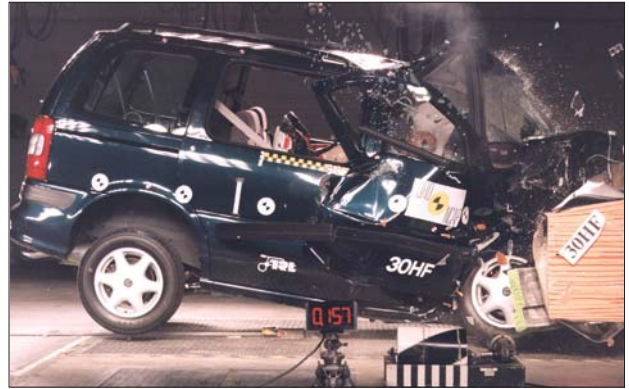
Intrusion of unstable passenger compartment allows the occupant to impact the interior
