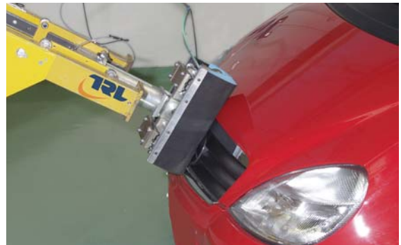
Upper Legform tests are used to assess the bonnet leading edge
