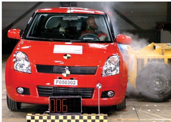
Side impact barrier test assesses protection, when hit by another car
