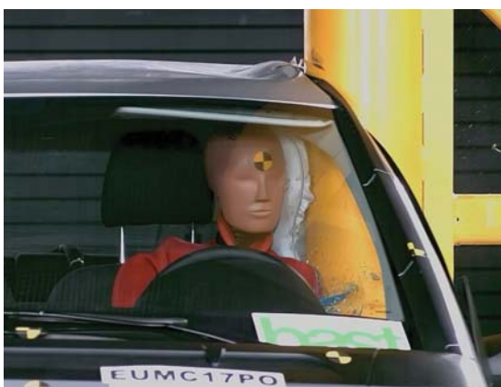
Pole test assesses the effectiveness of side impact head protection airbags
