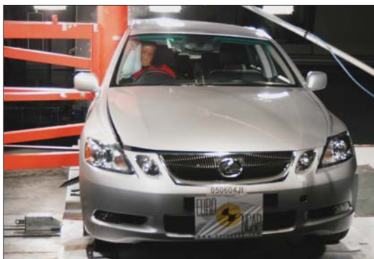
A pole test is added to assess side impact head protection (2000)
