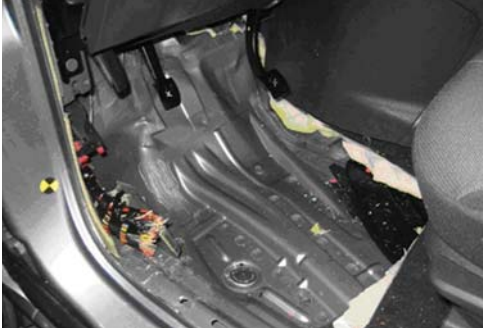
Prevention of footwell intrusion and control of pedal movement can help to protect the feet and ankles
