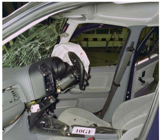
Impact with the steering wheel poses a serious risk to the driver
