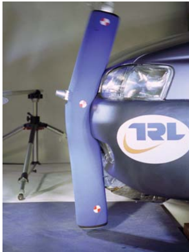
Legform tests are carried out to assess the bumper area
