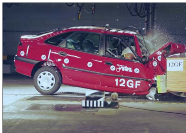
Head protection is compromised when the head slides off the airbag
