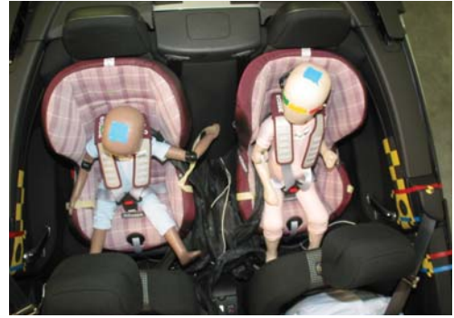
Child protection is assessed in the frontal and side impact barrier tests
