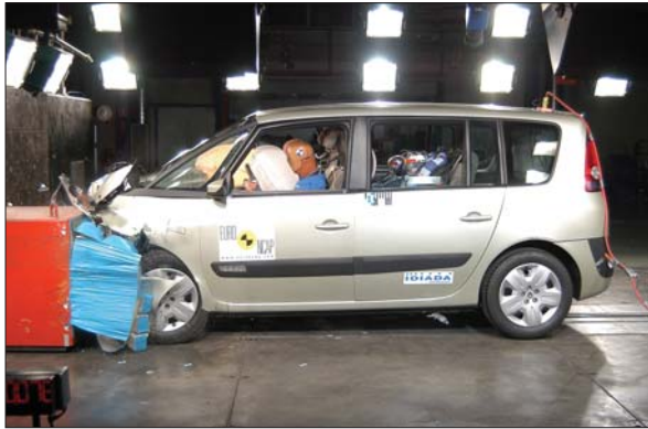
Frontal offset deformable barrier test at 64 km/h
